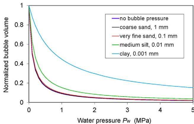
Fig. 4. Volumetric change in air bubbles with different diameters based on Boyle’s law with and without the effect of internal bubble pressure. The initial bubble diameter at zero water pressure was assumed to be 30% of the particle diameter of the materials shown.
