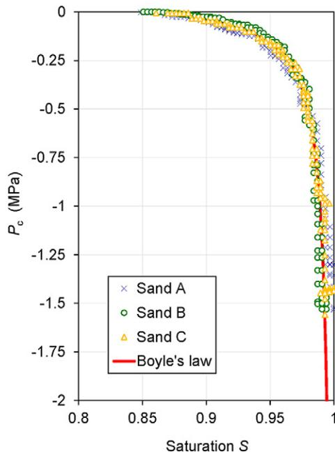
Fig. 6. Measured capillary pressure ( $P_c$ )–saturation ( $S$ ) data for three test sands. The red line is the theoretical estimation with  $S_{\text{max}} = 0.85$  based on Boyle's law without internal bubble pressure (Eq. [3]). The line coincides with the measured data.
