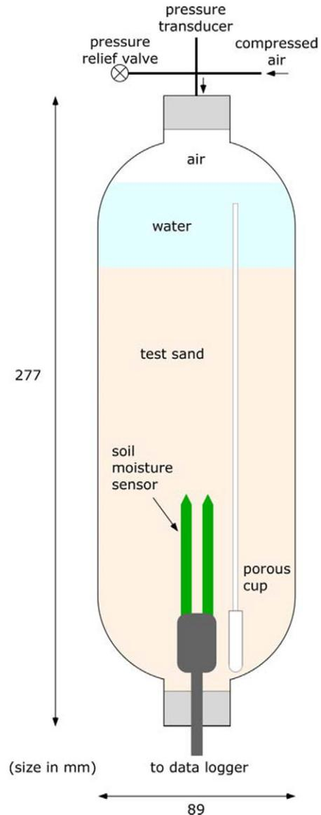
Fig. 3. Pressure chamber setup.
