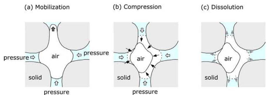
Fig. 2. Dominant mechanisms for saturation changes during the resaturation process: (a) mobilization of mobile bubbles, and (b) compression and (c) dissolution of immobile bubbles.
