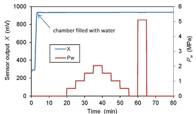
Fig. 5. Output values of the EC-5 soil moisture sensor under various water pressures  $P_w$ . No pressure dependence was observed.
