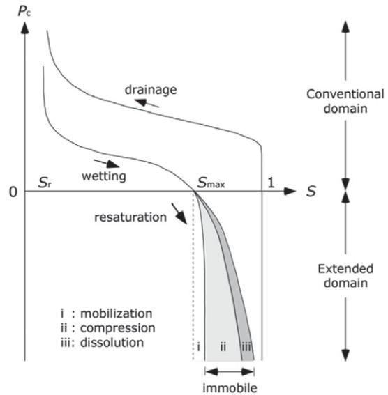
Fig. 1. Water retention curves in the conventional and extended domains. In the extended domain, contributions from three mechanisms (mobilization of mobile bubbles, compression and dissolution of immobile bubbles) are shown schematically.
