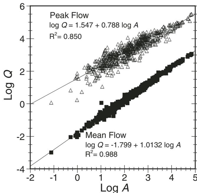
Figure 2. Log-log plot for discharge ( $Q$ ,  $m^3/s$ ) versus drainage area ( $A$ ,  $km^2$ ) for 550 USGS gaging stations in Pennsylvania. The linear relation for mean flow (squares) has a unit slope, so  $c = 1$ , but  $c \sim 0.79$  for maximum historic discharge (open triangles). A similar diagram for Missouri watersheds (Criss, 2003) also shows a unit slope for the mean flow relationship, but has  $c \sim 0.5$  for record flows. No data from either state suggest slopes greater than one.
