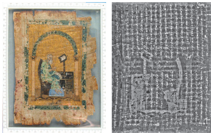
FIGURE 1 (LEFT) A leaf from the Archimedes Palimpsest covered by a forged painting from the twentieth century as viewed in normal light. (RIGHT) Image of the same page (reversed) and illuminated using synchrotron X-rays to stimulate X-ray fluorescence from the iron in the ink, which now shows the vertical Greek text written by the monk Myronas in 1229. PHOTO CREDIT UWE BERGMANN
