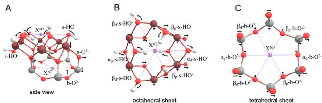
FIG. 5. PM7/COSMO optimized structure of the G1+ model for the exfoliated kaolinite.
