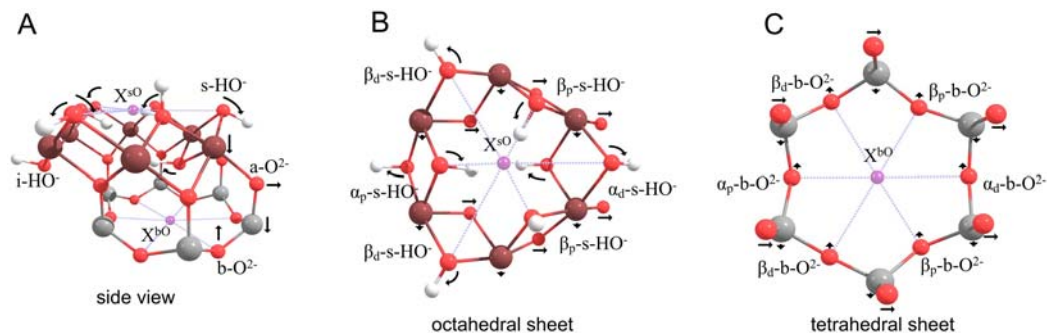
FIG. 3. B3LYP/TZVP optimized structure of the G1+ model for the exfoliated kaolinite.
