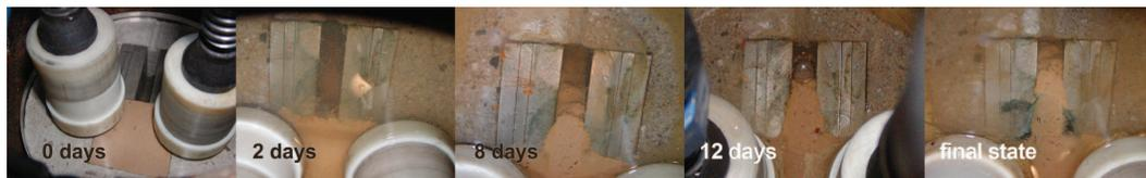
FIG. 4. The advance of bentonite into a fissure.
